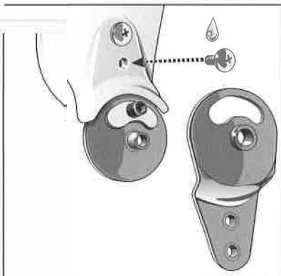
7. Insert hinges and assemble to AFO by securing #8-32 hinge attachment screws with threadlock. If required, careful peening of the #8-32 attachment screws will ensure permanent fixture in final assembly.
