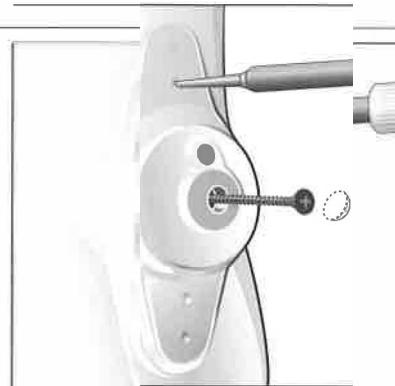
5. Stretch an interface nylon over the model and vacuum form to standard procedures. After thermoplastic has cooled, grind the plastic over the center axis screw head and remove plaster screws. "Hot mark" the center of each attachment hole before removing the AFO shell. Mark and cut trim lines to release AFO from cast.
