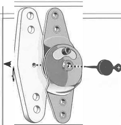
3. Fit the precut pelite fabrication blanks to the hinge. Remove the center axis screw and replace with the black plaster screw and washer. Carefully thread screw through the center axis and pelite blank.
