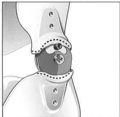
6. With the hinges removed, drill a #18 hole through "hot marks" centered at all clearance hole locations on the plastic. **Do not oversize clearance holes.**
