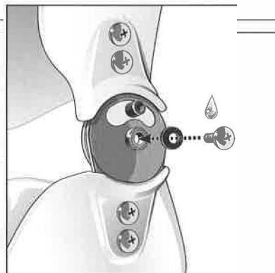
8. Place S.S. washer under the center axis screw head and torque the screw to 3-5 inch pounds.
