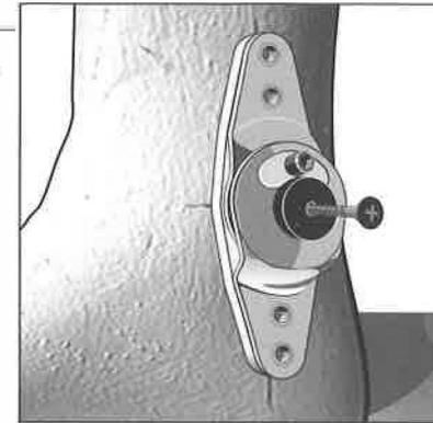
4. Drill 1/16" pilot holes at the joint axis on medial and lateral sides of plaster model. Align joints to the vertical lines, attaching hinges by tightening plaster screws until joints are flush with the cast surface.
