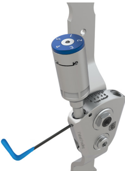
Figure 1. Unlock / lock the ROM Adjustment using the 1.5mm hex wrench to loosen / tighten the ROM Lock Set Screw.
