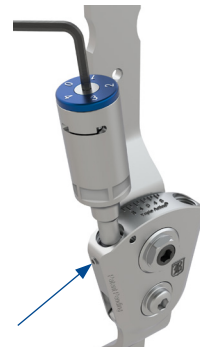
Figure 3. Loosen the ROM Dial screw using the 2mm adjustment wrench and zero the ROM setting by turning the blue ROM dial. The ROM lock set screw serves as a reference for this adjustment.
